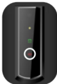
**19\*** *The red light indicates that the phone battery is being charged, while when it turns off indicates that the charging has been completed.*
