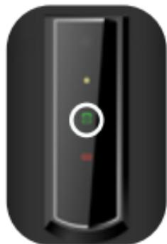
**18\*** *Flashing green light indicates an unread call or SMS. This will turn off only when the missed call or the unread SMS is checked*
